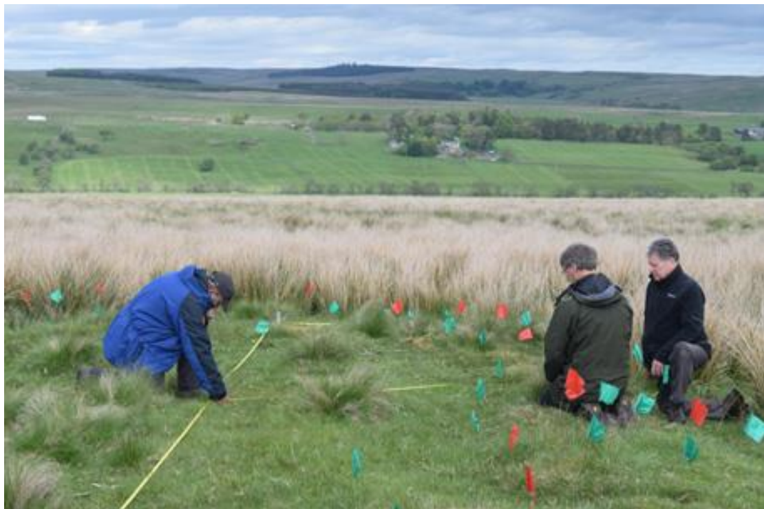
Fig.11 Tape and offset measurement at R09
